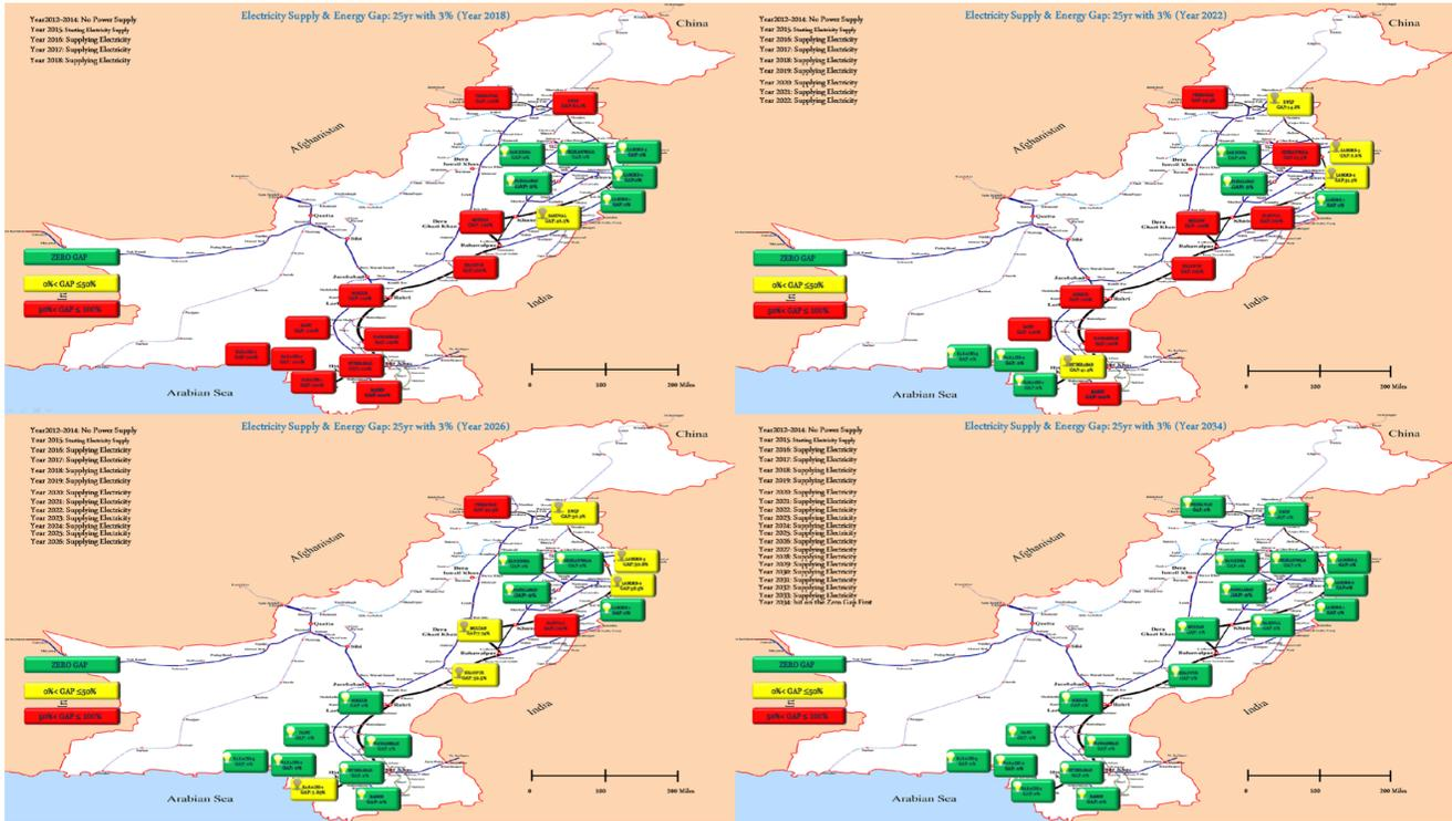
Figure 9: The optimal solution on transmission and energy gaps at demand zones for the scenario with 5% demand growth, a budget of 3% GDP and a 25-year planning horizon. Green - 0% gap, yellow - 1% to 50% gap, red - 51% gap and above.
