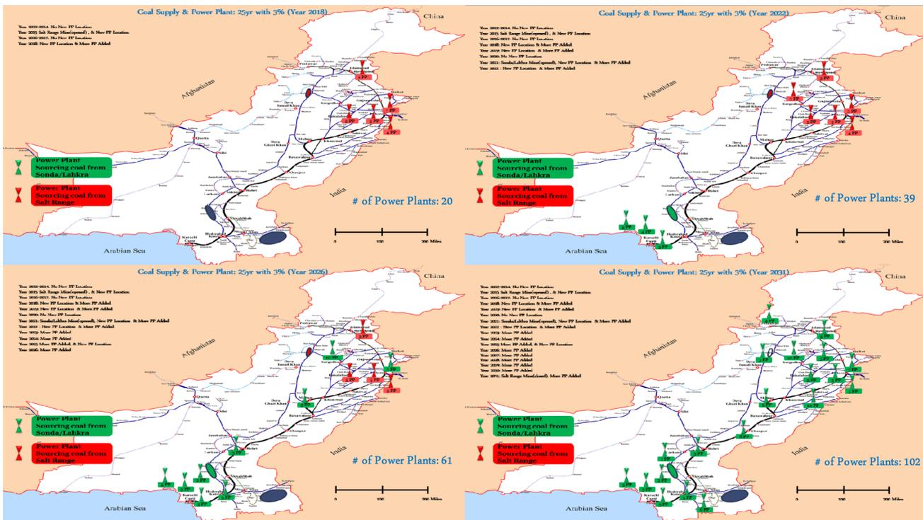
Figure 8: The optimal solution on reserve selection and power plant locations for the scenario with 5% demand growth, a budget of 3% GDP and a 25-year planning horizon. Circles - coal reserves; empty circles - reserves that run out; collate shapes - power plants (the box below indicates the number of power plants in service).
